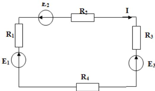
$$I = \frac{E_1 - E_2 - E_3}{R_1 + R_2 + R_3}$$
