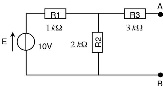
$$R_N = R_3 + \frac{R_1 R_2}{R_1 + R_2} = 3,67 \text{ k}\Omega$$
