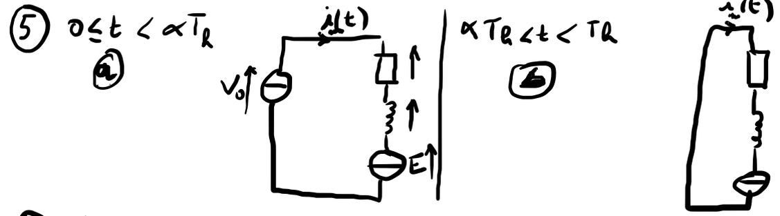
⑥ phase a :  $V_0 = R i_m(t) + L \frac{d i_m(t)}{dt} + E$
